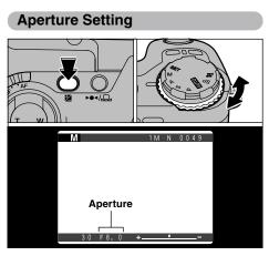
Set the aperture by holding down the "\overline{\mathbb{Z}}" (exposure compensation) button and turning the Command dial.
